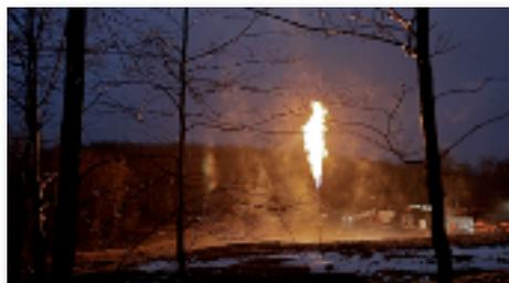
Flaring takes place after a gas well has been drilled and before it is put into operation.
