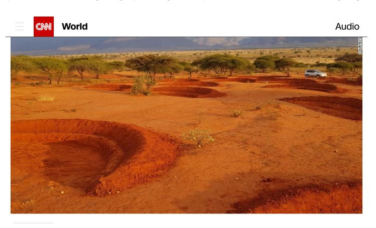
Semi-circular shaped bunds trap water running off the ground and allow it to penetrate the earth. Grass seed sown inside the bunds grows, and over time greenery extends beyond the bund.
